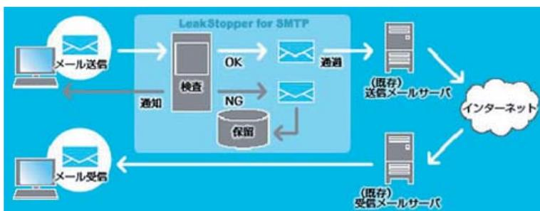
図1 LeakStopper for SMTP設置例
